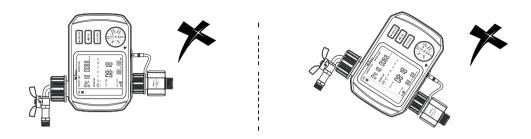
Tips: If the connection between the timer and the faucet or hose is not tight or leaking occurs, wrap more Teflon Tape (Thread seal tape) to make them tight.
