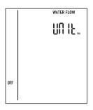
Step 1: Turn the dial to OFF, and press and hold the ★/OK for 2 seconds. The screen will display the characters WATER FLOW and UNIt (UNIT) and the unit parameter of the water flow meter will flash.
