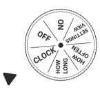
Step1: Turn the dial to CLOCK, and the hour of the current time will flash. Press the +/DELAY or -/LOCK to adjust the number, then press the //OK to confirm.
