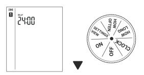
Step 1: Turn the dial to **ON**, press and hold the +/DELAY for 2 seconds, and the screen will display the character DELAY and the related delay time.
