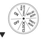
Turn the dial to **OFF**, the screen will only display the character **OFF**, and the timer will stop all watering plans and actions.
