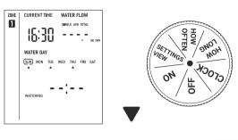
Step 2: Press the +/DELAY or -/LOCK to adjust the watering time.
