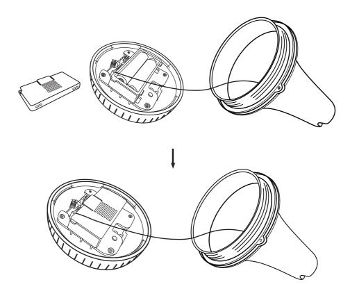
. Make sure the silicone waterproof ring is well placed, then close and tighten the lid of the pool thermometer.
